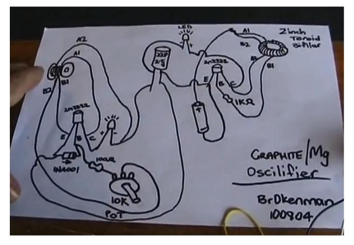
Upper Right hand of pic is the Joule Theif, which uses an LED as a Load (The LED was replaced with a 1N4004 Diode) the current than runs to a 22 farad 2.5 volt SuperCap
